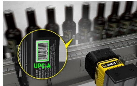
Read UPC-A codes on curved surfaces
