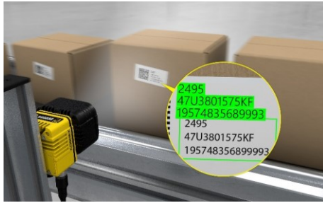
Read multi-line text on printed labels
