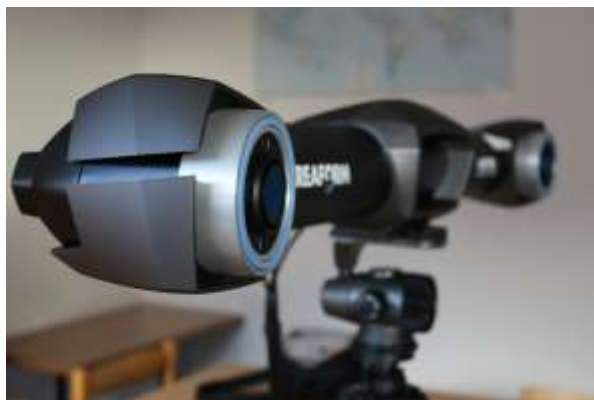
MetraSCAN 350 - skener + tracker
