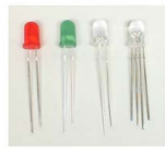
Figure 2-1: Discrete LEDs, from left to right: standard red and green, high-efficiency in various colors, and RGB.
