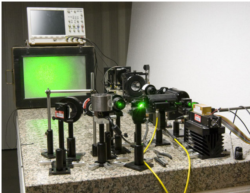
Figure 5.3: Digital holographic interferometry (DHI) measurement setup and realization; (a) Scheme of the glass plate surface displacement measurement using the DHI method.; (b) The photograph of a realization of the experimental setup of the glass plate surface displacement distribution measurement using the DHI method.
