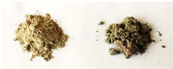
Figure 2: Homogenized bentonite on the left and raw (unhomogenized) bentonite on the right.
